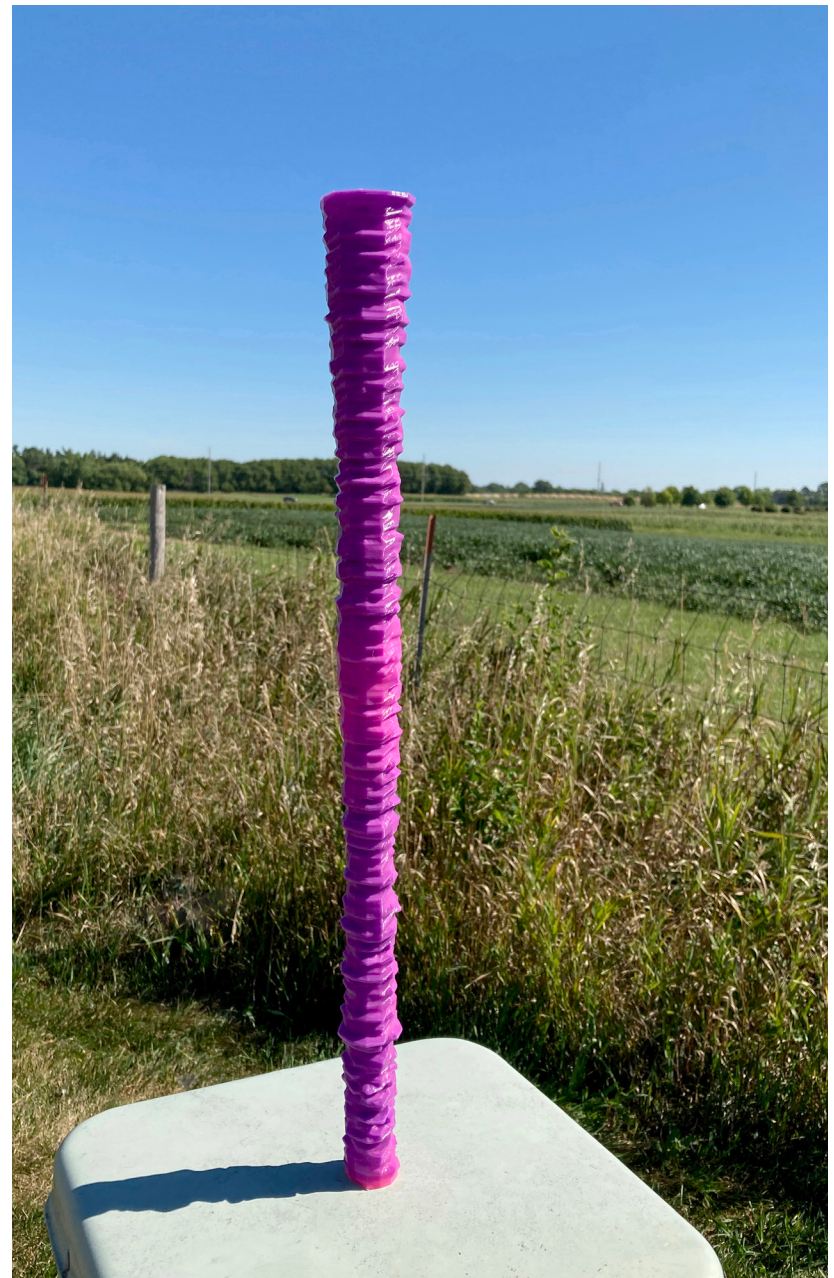
Material: 3D printed PLA (Polylactic acid), Dimensions: 2 X 2 X 21.75 in
